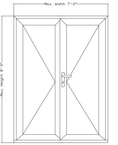
Max. Width for French Entry Door is 86" Max. Width for French Balcony Door 86"
