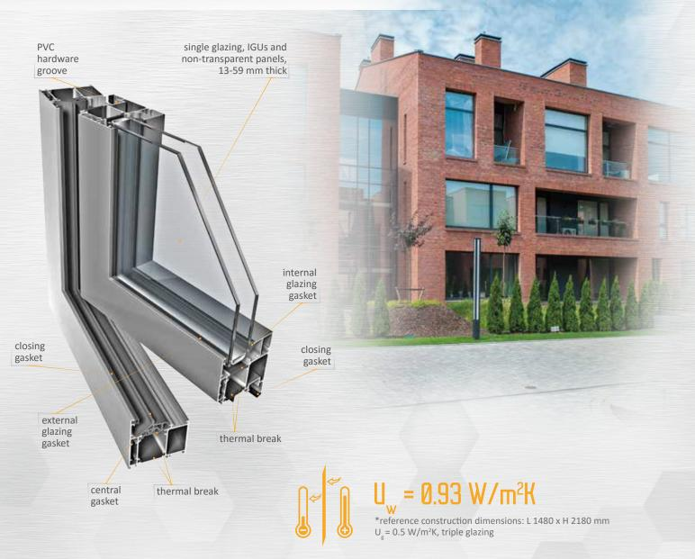
An insulated aluminium profile system with the Euro hardware groove as well as the PVC hardware groove in window sash profiles featuring very high thermal performance.
