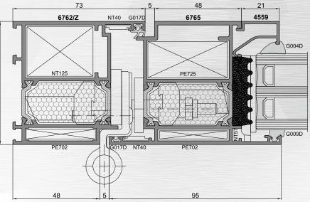
An insulated, three-cavity profile system designed for the construction of doors.
